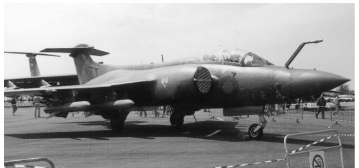
Fig 3-2 Area Rule- 'Coke-Bottle' Fuselage
