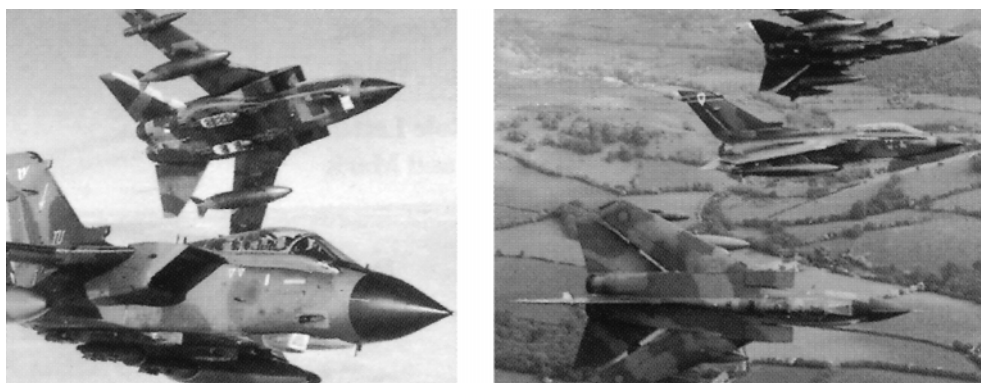
Fig 3-4 Variable Sweep-Back (Tornado)
